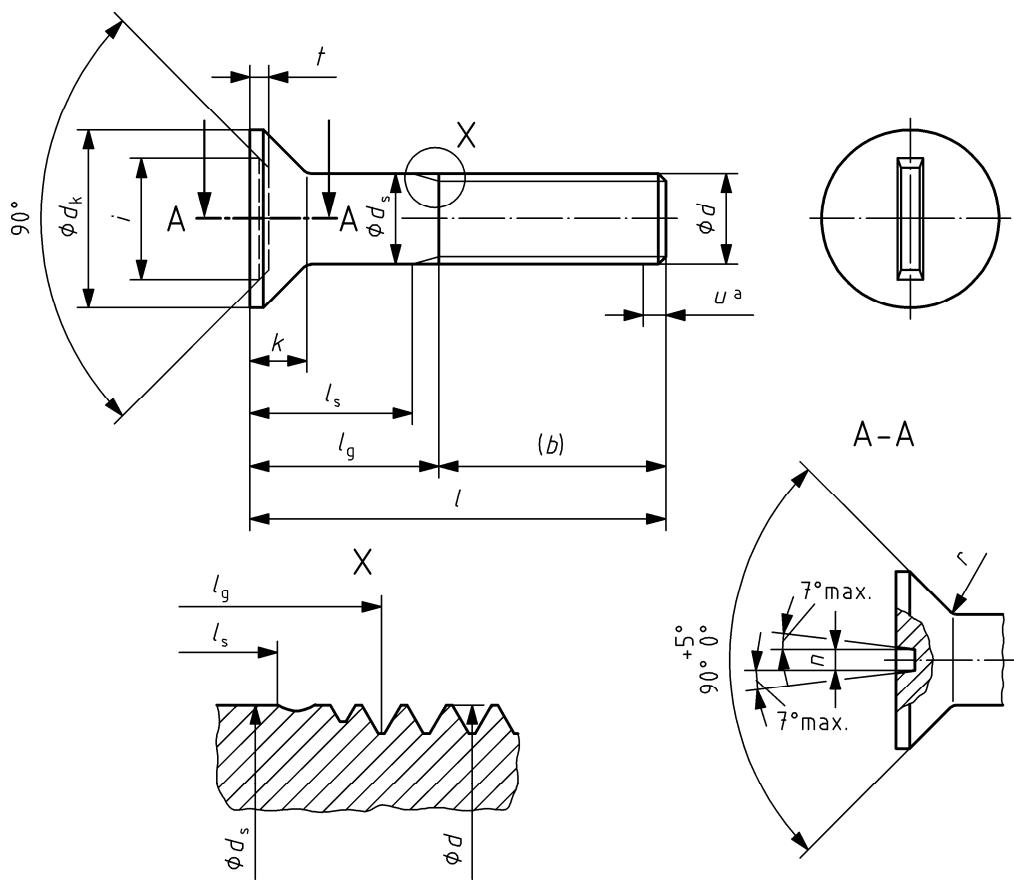
The difference between  $l_g$  and  $l_s$  shall not be less than  $1,5 P$ .
